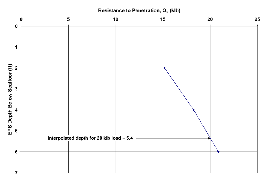
Figure 8.4-2. Plot of predicted soil resistance to EPS penetration.
